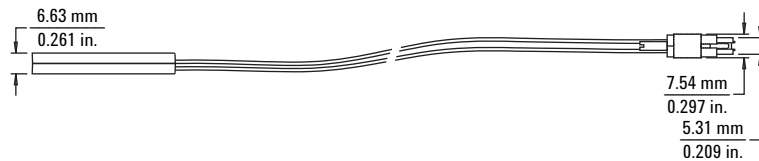
Figure 3.6. E5394A and E5396A soft touch probe dimensions
